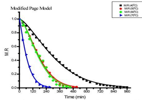
Figure 2. Moisture ratio vs drying time in modified Page model
