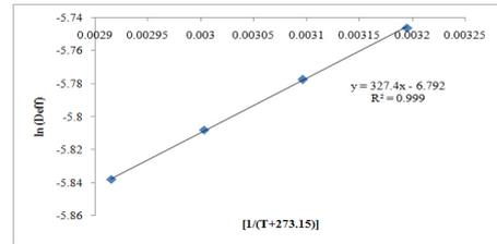
Figure 4. Logarithmic of effective moisture diffusivity vs function of the inverse of absolute Temperature in K
